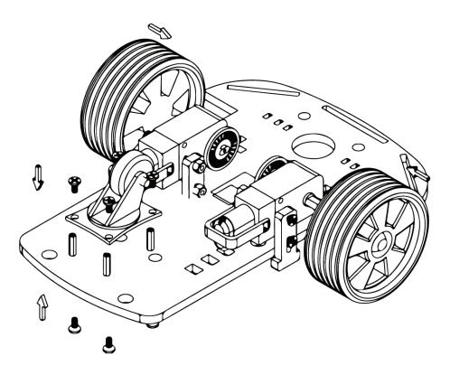
Now mount the mounting plate with the help of the enclosed mounting plate kit. The according mounting holes for Robot05 are marked on the mounting plate as **R1**.
