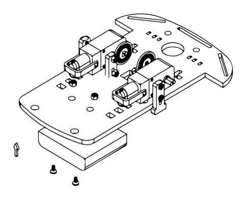
Put in the spacers and mount the front axle.
