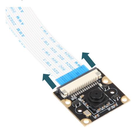
Next, you can now simply remove the ribbon cable and insert the appropriate ribbon cable for the Raspberry Pi 5 and **push the clip in the opposite direction of the arrows shown above to reattach the ribbon cable.**
