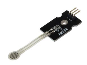
This pressure sensor works by means of analog resistance detection, when external pressure is applied to the sensor, the resistance and thus the voltage of the analog signal changes. The sensor is highly sensitive, and the sensor strip is waterproof and flexible.
