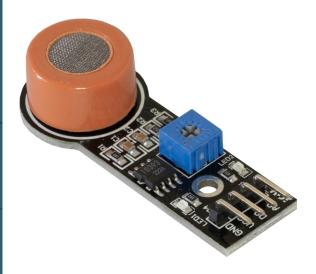
This analog gas sensor has a small heating part with an electronical chemical sensor. It is suitable for indoor usage. The sensor can output exact values only after warmup phase.
