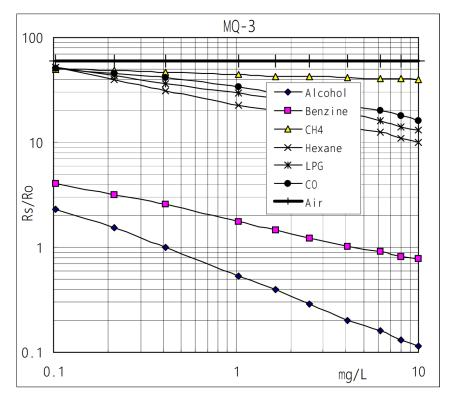
This shows the typical sensitivity characteristics of the MQ-3. Rs means resistance of the sensor in different gases, Ro means resistance of sensor in 1000ppm Alcohol.
