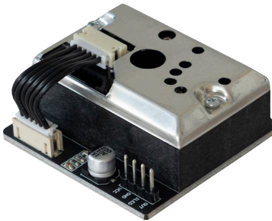
The GP2Y1014AU is an optical sensor for the detection of dust particles. The light reflected by the dust is detected by an integrated infrared diode and a phototransistor and can thus be determined in an analog value.
