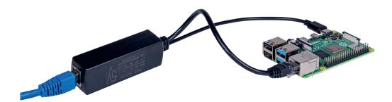
Attention! The device is suitable for network speeds up to 100 Mbps. For higher network speeds, you must limit the speed of your Raspberry Pi to 100 Mbps using the following command:
