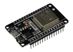
With the NodeMCU-ESP32, comfortable prototyping is possible with simple programming via Lua script or the Arduino IDE and the breadboard-compatible design. This board has 2.4 GHz dual-mode Wifi and a BT wireless connection. In addition, a 512 KB SRAM and a 4MB memory are integrated on the microcontroller development board. The board has 21 pins for interface connection, including I2C, SPI, UART, DAC and ADC.
