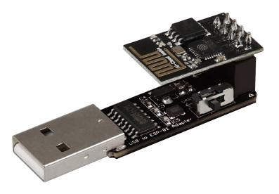
Next to the yellow connector is a small switch (also shown in the picture). Note that the switch should be on **Prog** if you want to program your ESP8266. For the regular use, you must set the switch to **UART**.
