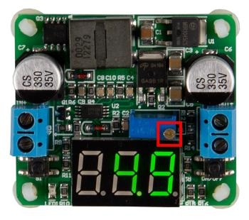
With the **S1** button you can switch through a total of three display modes. The factory setting automatically shows the input mode after starting the device. Here, the input voltage is shown on the display. The LED, which is located directly below the button, lights up permanently.
