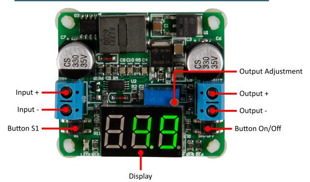
The freely configurable voltage transformer module is equipped with a "Step UP" and a "Step DOWN" function. The voltage can be set individually by means of a trimmer and is shown on the integrated segment display.
