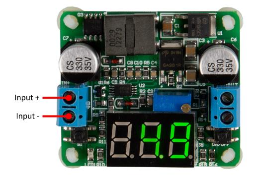
Next, connect the cables of the device to be supplied to the output (**Output + / Output -**). The voltage converter is now ready for use.
