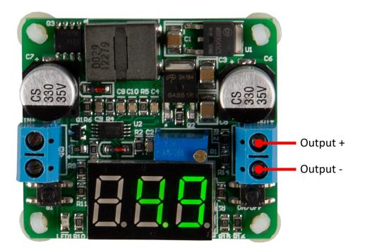
The desired voltage can be set with the adjustment screw. The display shows the current output voltage.
