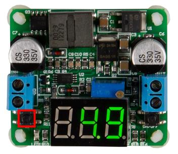
With the ON/OFF key, the voltage output can additionally be switched on or off.
