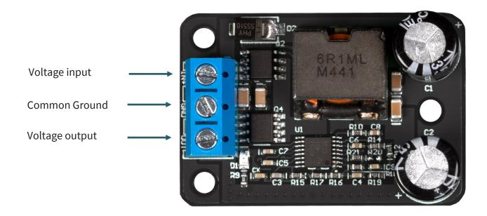
ATTENTION: The board gets hot under load! We recommend additional cooling of the board for high loads. Our information and take-back obligations according to the Electrical and Electronic Equipment Act (ElektroG)
