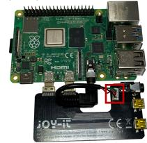
4. Now place the Raspberry Pi with the circuit board on the bottom of the case.
