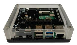
7. Connect now the fan, which is attached at the cover, to the big board. Make sure that the red cable is connected to "+" and the black cable to "-".
