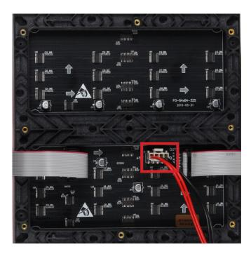
Up to three matrices can be operated parallel while using the 40-pin GPIO strip of the Raspberry Pi. Additional matrices can be connected in series to each matrix. Please make sure to adjust your power supply accordingly.
