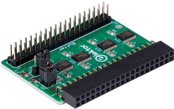
This logic level converter board allows operating devices with a logic level of 5 V at the 40-pin GPIO header of the Raspberry Pi. The logic level of the GPIOs can be switched between 3.3 V and 5 V with a jumper.
