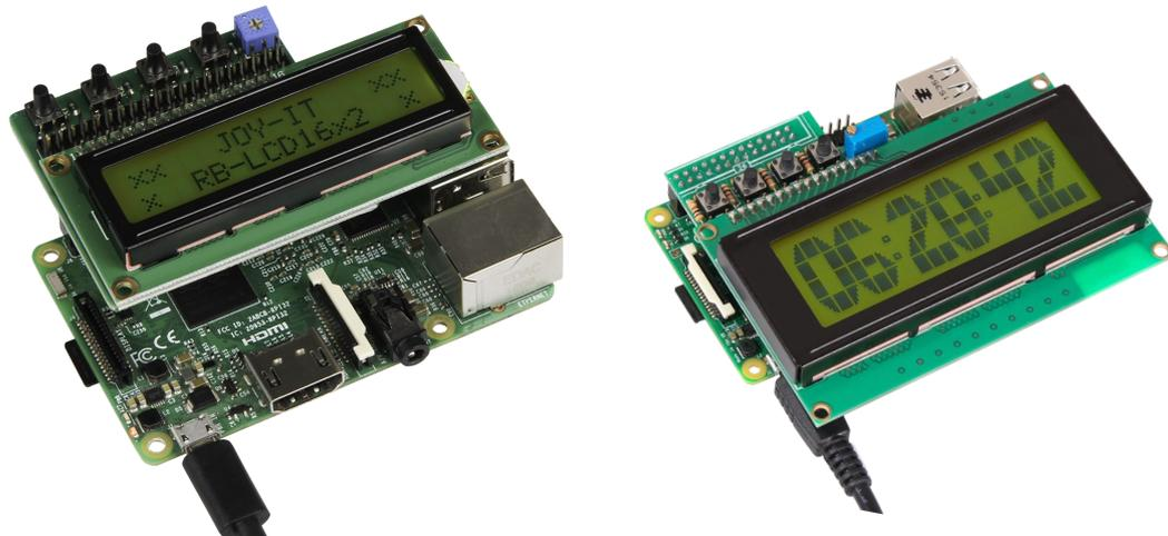
The buttons are connected to the GPIOs of the Raspberry Pi. The backlight is permanently activated on this display and cannot be switched off.
