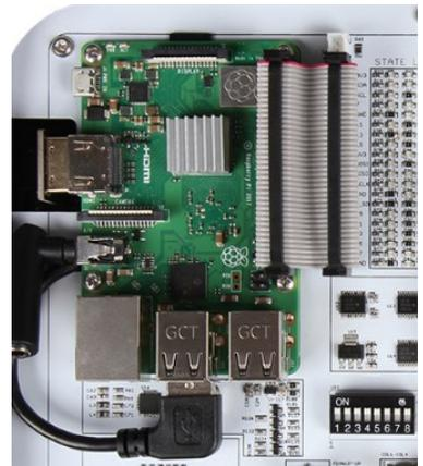
Now plug the USB cable into one of the USB ports and connect the GPIO bar of the Raspberry Pi to the one on the Joy-Pi, using the supplied cable.
