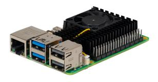
Discover the next generation of cooling technology for the Raspberry Pi 5 with our active cooling unit. This state of the art cooling solution has been specifically designed for the Raspberry Pi 5 and offers a more reliable and stable mounting compared to traditional clip-on systems thanks to its robust screw mounting.
