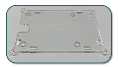
Now place your Raspberry Pi on the base plate. Make sure that the SD card slot is above the notch of the base plate.
