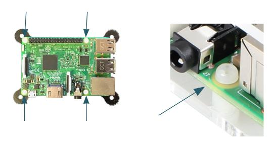
Finally, screw the brass spacer tight at the bottom and the top.
