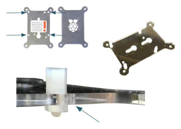
Now you can put the Raspberry Pi onto the spacers and screw it tight with four synthetic screws.
