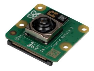
The Raspberry Pi Camera Module 3 is a compact camera for the Raspberry Pi, equipped with a 12 megapixel Sony IMX708 sensor.
