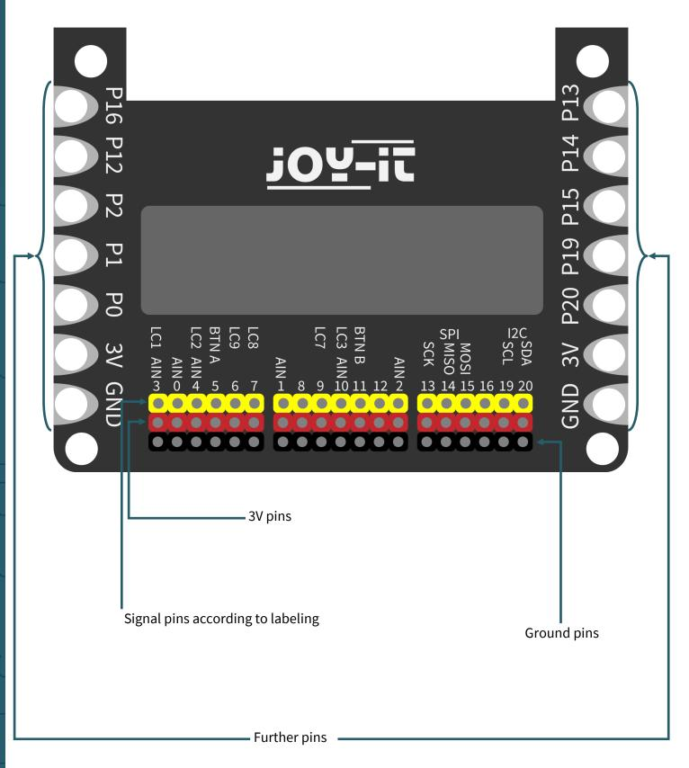
AIN - analog input LC - LED column BTN - Button A and B
