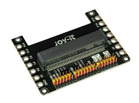
This sensor shield helps you connect multiple sensors to your micro:bit. All IO pins are routed out via the 3-pin interfaces, each together with a GND and 3 V pin. This makes it easy to connect circuits with jumper wires. You can also connect the supply voltage for your micro:bit to the 3 V and ground pins via the breakout board.
