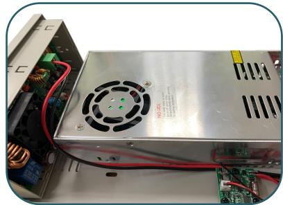
9. The RD6006-NT has a switch with which you can set the input voltage to 110 or 230V.
