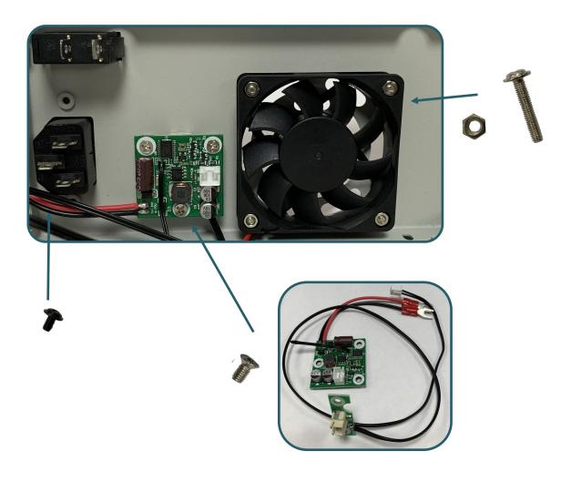
3. Now, mount the power supply into the case. Therefore, you have to screw it from the bottom of the case with the big silver screws.
