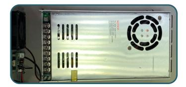
4. Now, connect the fan to the fan controller and the fan controller to the power supply. Therefore, connect the black cable of the fan control to the power supply with one of the anticipated terminals V- and the red cable with one of the V+ terminals.
