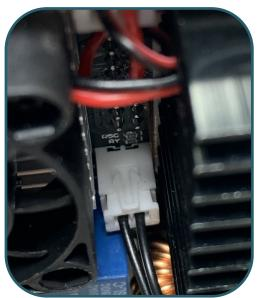
8. The RD6006-NT has a switch with which you can set the input voltage to 110 or 230V.
