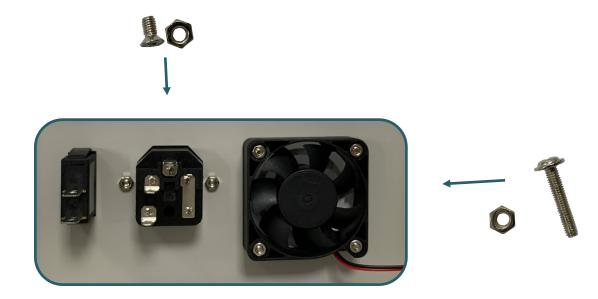
4. Now, mount the power supply into the case. Therefore, you have to screw it from the bottom of the case with the big silver screws.
