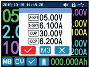
Press **SHIFT + I-SET** or **SHIFT+ V-SET** keys to set the overcurrent protection/overvoltage protection limit. The operation is identical to the setting of the output current.
