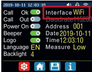
As an alternative to the USB connection, the laboratory power supply can also be controlled by the radio module via WiFi. For control via WiFi, the corresponding interface must first be activated on the device. To do this, open the settings by pressing **SHIFT** and **0** and set the interface option here to **WiFi**. Please note that the changes will only take effect after restarting the device.
