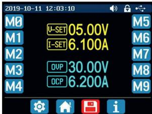
Press **SHIFT + 0** to enter the system settings menu. Now press the right arrow key twice to call up the settings menu for data storage. Use the direction keys to select the desired data group.
