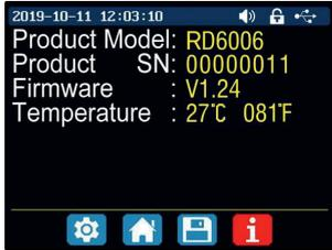
Open the system settings menu (**SHIFT + 0**) and press the right arrow key three times to enter the system information menu. Here you will see the model number, the serial number, the current firmware version, and the current system temperature.
