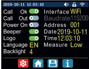
Press **SHIFT + 0** to enter the system settings menu. The desired setting can be selected using the direction keys. The current selection is highlighted in red. The setting can be changed by pressing the encoder.
