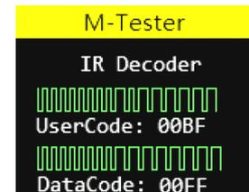
However, **only** the NEC protocol (which is used by many manufacturers) can be decoded.
