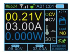
If the load current reaches the set current, the output is at the same level as the set current and constant current. Then the CC light comes on. If the load current is below the set current, the output is a constant voltage. The CV light comes on.
