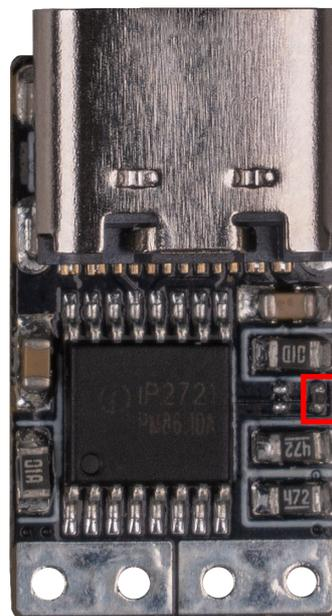
Right resistor soldered = 20 V
