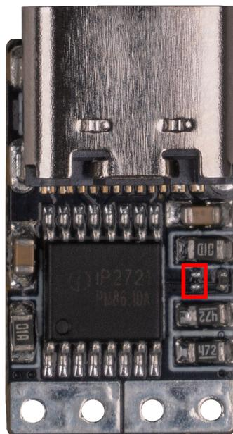
Left resistor soldered = 5 V
