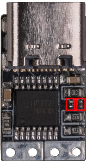
Both resistors soldered = 5 V
