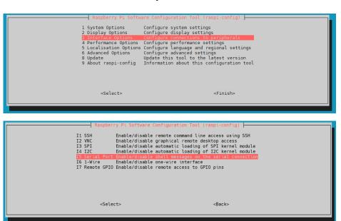
Now deactivate the serial login shell and activate the serial hardware.
