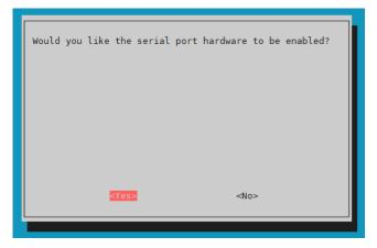
You have now enabled serial communication on your Raspberry Pi. Now restart your device once to apply the changes. Make sure that the serial library is installed on your Raspberry Pi. To do this, run the following command in your console.
