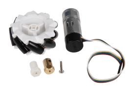
This omni wheel and motor kit is a full set of 4 high-quality omni wheels with matching motors and mounting screws.
