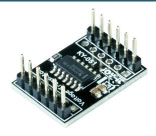
This module converts digital signals from one voltage down to another or up. This makes it possible to operate sensors and modules that work with 5 V logic with 3 V systems, such as the Raspberry Pi, and vice versa.
