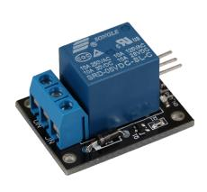
With the relay you can switch higher voltages by using a 5V output. This module can be soldered solidly or can be plugged on a breadboard.
