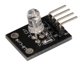
The LED module contains a red, blue and green LED. These are connected through a common cathode. In total, 16.7 million colors can be depicted.
