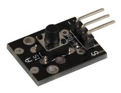
This tough button module is perfect to use in your venture or your experiment. It can be soldered solidly or can be plugged on a breadboard.
