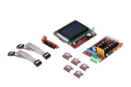
This set builds your basic module for the installation of your own 3D printer on the basis of Arduino. With the fitting installed software on the Arduino Mega, it can show you the current status or rather information like temperature on the included LCD-display.
