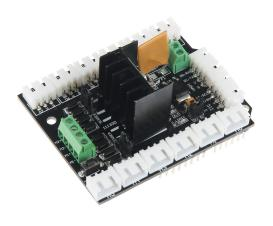
This Motorshield can be clipped on directly to the Arduino L298N chip for DC motors or 2-phases and 4-phases stepper motors.
