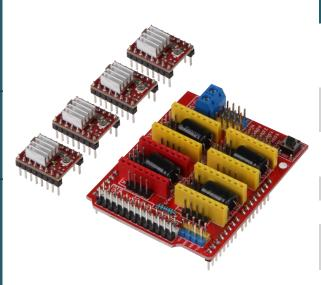
With this expansion board, which is made for use with an Arduino Uno or Arduino Uno compatible board, you can install a custom CNC router. It can be powered from 12 to 36 volts depending on your needs. Control with the four included A4988 motor drivers operates up to 4 axes and is lightweight as it is 100% GRBL compatible.
